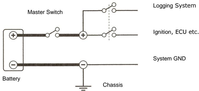
**Figure 6** - Battery Connections
