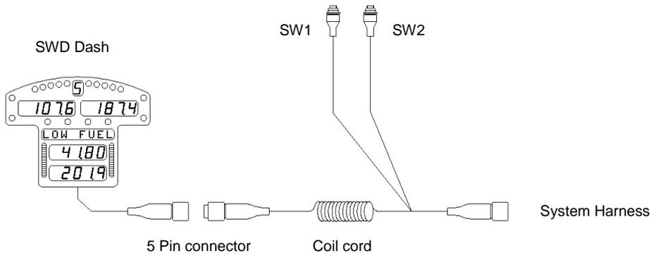
**Figure 15** - Typical SWD installation
