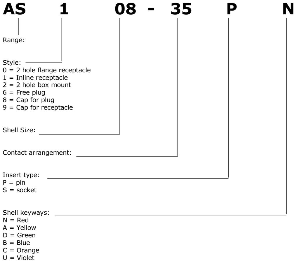
**Figure 5** - Connector Part Numbering
