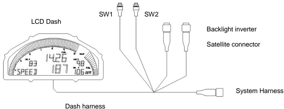
**Figure 17** – Typical LCD Installation
