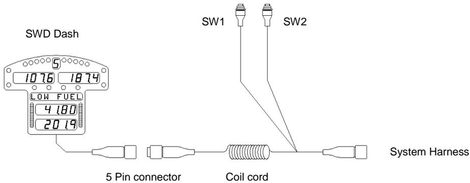
**Figure 15** - Typical SWD installation
