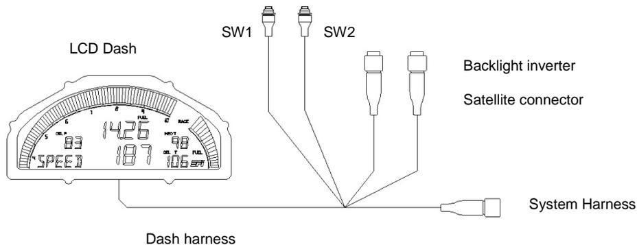
**Figure 17** – Typical LCD Installation
